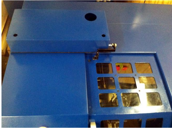
The automatic shield opener, in closed position
